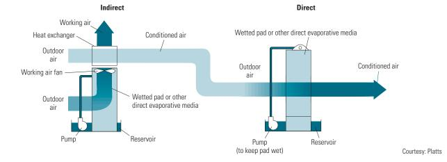
Dry air leaving the indirect stage can be further cooled in the direct stage to a temperature below the outdoor wetbulb temperature. The darker-colored arrow indicates that moisture has been added to the airstream.
