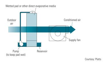
going, an equal quantity of air must constantly be exhausted from the building to offset the inflow. The chief drawback of direct coolers, at least in moist climates, is that they increase the humidity of the conditioned space.
