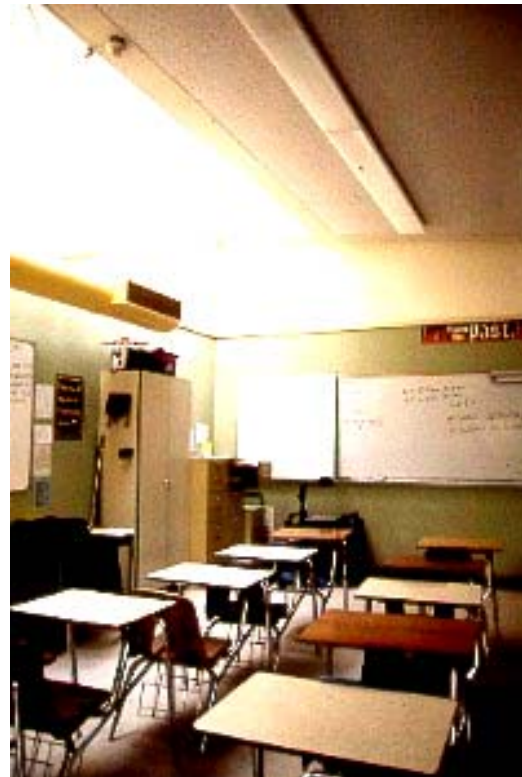
Skylit wall wash delivers daylight across two-thirds of this classroom. Lisa Hescong, photographer.
