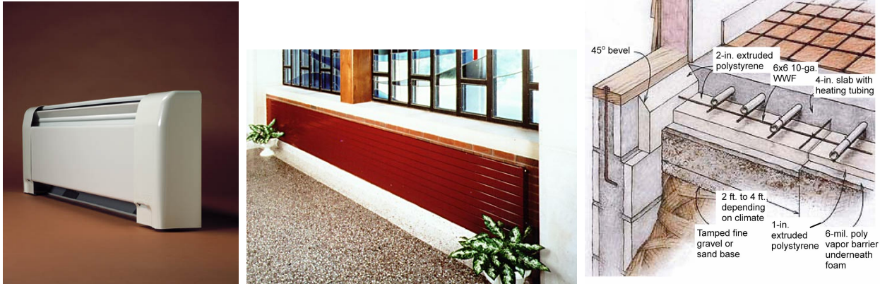
Figure 135—Examples of Hydronic Heating-Only System Options
