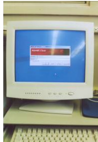
Figure 46—Veiling Glare from Luminaires on Computer Screen
