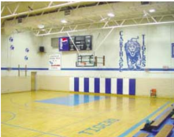
Figure 55—Gym with fluorescent high bay T-5 luminaires.
