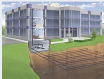
Horizontal Loop System
