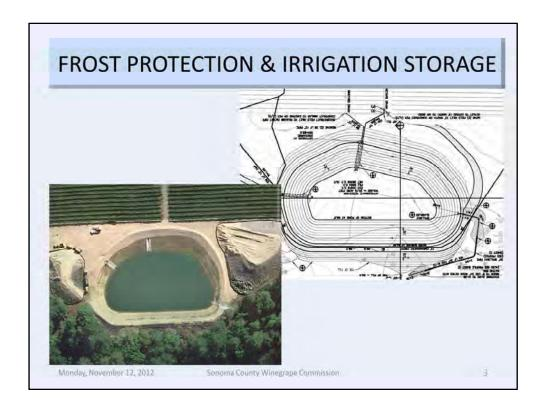
Siting this pond below the existing vineyards provided for gravity collection from surface runoff and vineyard sub-drains.
