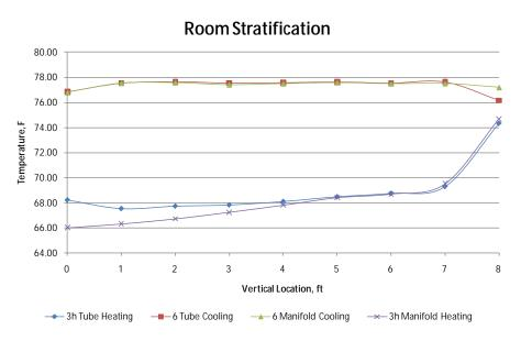
Figure 71: Temperature Stratification with Radiant Panels
