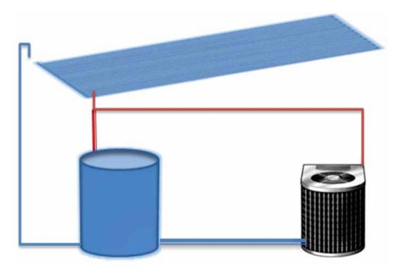
Figure 1: Panel, Chiller, and Storage Tank Schematic
