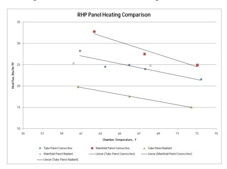
Figure 70: Convective vs. Radiant Heating Performance
