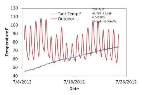
Figure 53: Tank Heat Gain with System Off
