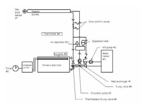
Figure 27: System Layout Schematic
