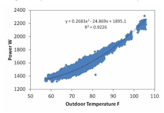
Figure 56: Compressor Power Draw as a Function of Outdoor Temperature
