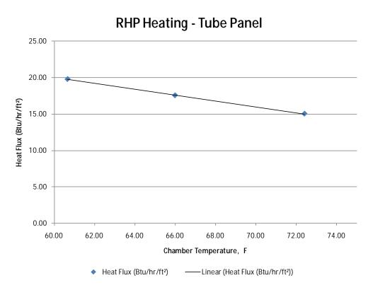
Figure 68: Effect of Water Inlet Temperature on Heat Flux for the Tube Panel in Radiant Heating Mode
