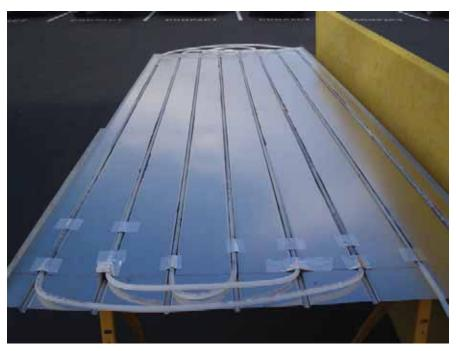
Figure 16: Serpentine Tube Panel
