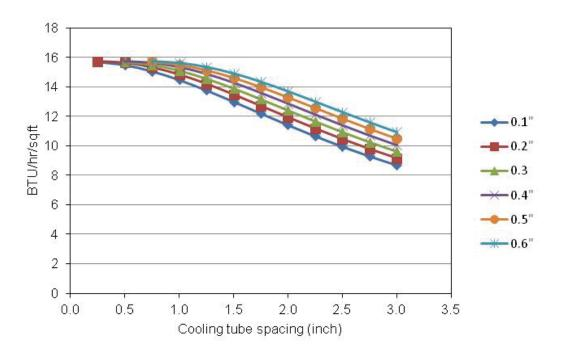
Figure 12: Btu per Dollar as a Function of Tube Spacing For Various Tube Diameters
