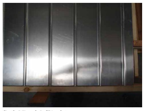
Figure 17: View of the Underside of the Serpentine Tube Panel
