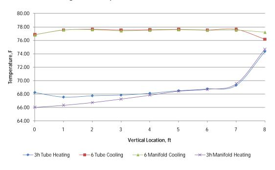
Figure 26: Temperature Stratification with Radiant Panels
