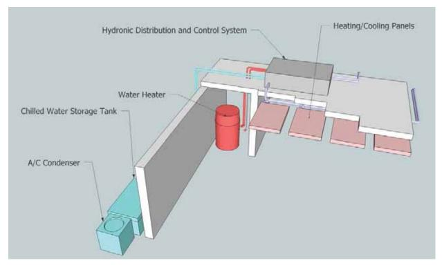
Figure 80: System Schematic
