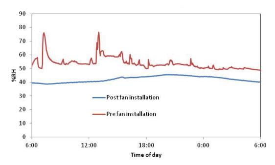
Figure 51: Typical Bathroom Humidity Levels At 6th Ave Pre and Post Fan Installation
