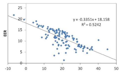
Temperature difference between tank and outside air
