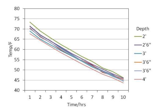
Figure 22: Tank Cooling Profile
