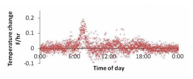
Figure 54: Tank Temperature Rise Plotted Vs. Time of Day with the System Off
