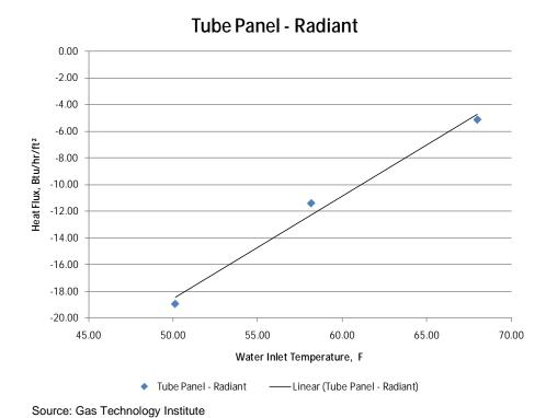
Figure 25: Radiant Cooling Heat Flux for Tube Panel with Varying Water Flow Rate
