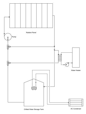
Figure 57: Preliminary HVAC System Design
