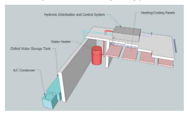
Figure 37: Schematic of Radiant Heating and Cooling System
