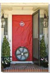
Fig. 9.3 Blower door testing its repeated periodically during air sealing operations to provide leadback to the crew about their progress towards their air sightness target.
