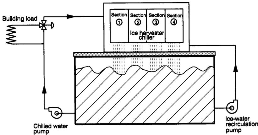
Figure 3. Typical ice-harvesting configuration.<sup>(b)</sup>
