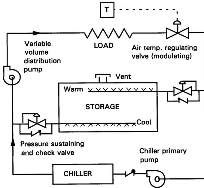
Note: Tank water level is above chiller and distribution pumps and below highest system piping.
