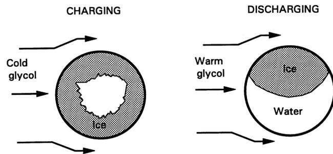
Figure 10. Encapsulated ice balls.<sup>(d)</sup>
