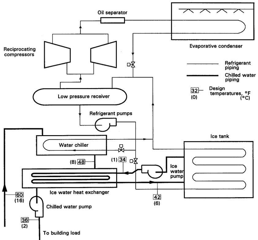
Figure 6. Direct refrigerant external-melt ice-on-coil configuration.<sup>(c)</sup>
