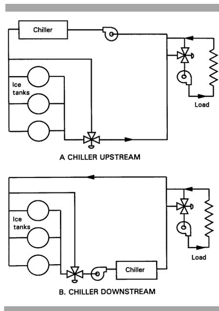
Figure 15. Upstream and downstream chiller configurations.<sup>(f)</sup>
