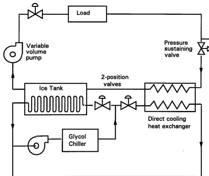
Figure 7. Secondary coolant external-melt ice-on-coil configuration.<sup>(c)</sup>
