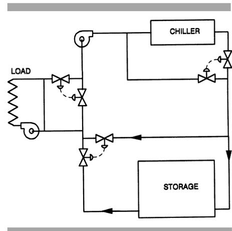
Figure 11. Typical encapsulated ice configuration.<sup>(d)</sup>
