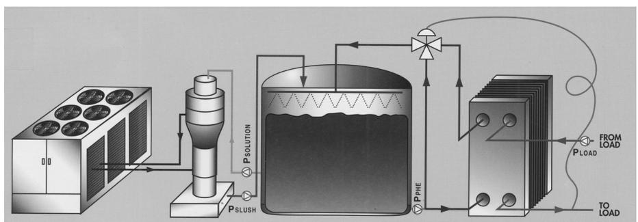
Figure 9. Typical ice slurry configuration.<sup>(d)</sup>
