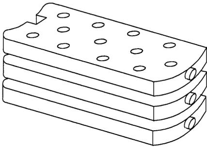
Figure 12. Eutectic salt containers.<sup>(e)</sup>
