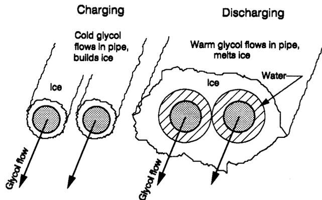
Figure 5. Internal-melt ice-on-coil.<sup>(b)</sup>
