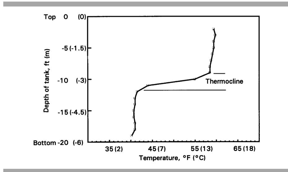
Figure 1. Chilled water stratification.<sup>(a)</sup>
