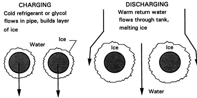
Figure 4. External-melt ice-on-coil.<sup>(b)</sup>
