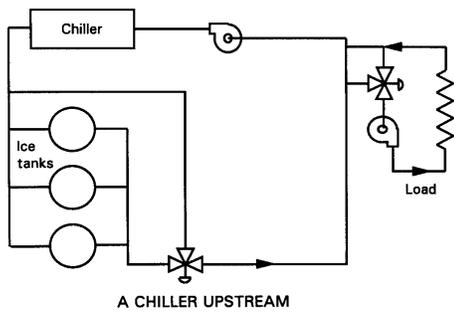
Figure 8. Typical internal-melt ice-on-coil configuration.<sup>(d)</sup>
