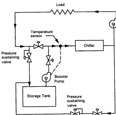
Figure 13. Typical eutectic salt configuration.<sup>(e)</sup>
