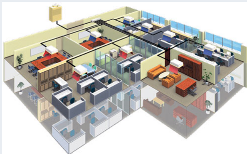
VRF System with One Condenser Serving Multiple Room Units
